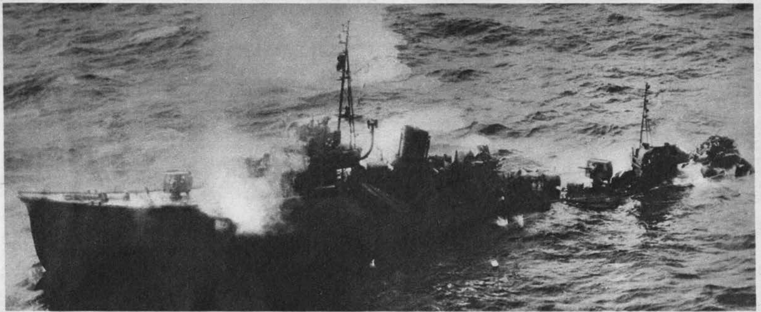
Sinking by the stern , Chidori-Otori TB still displays its low profile. Weight of ship (trunked stack, elementary bridge) is pushed forward,
